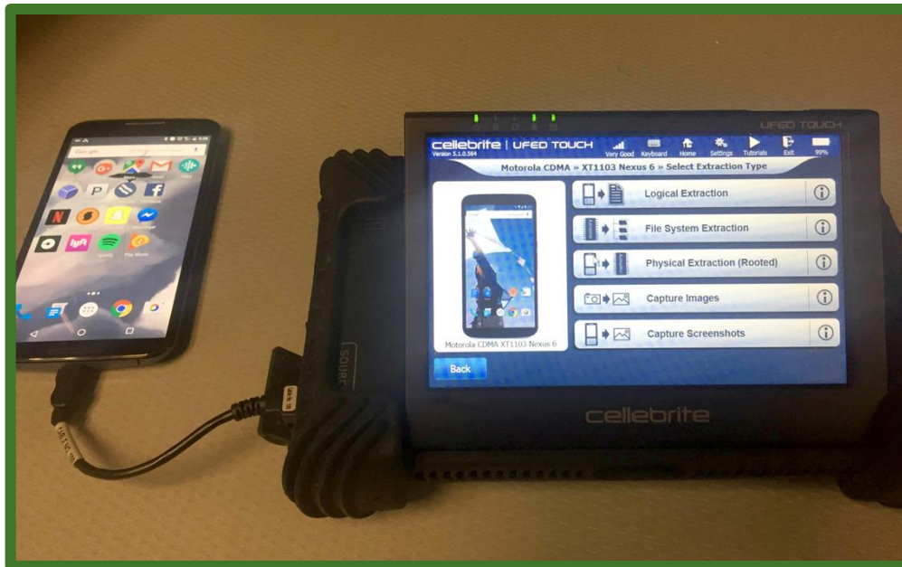
Figure – An early model of Cellebrite UFED used by HTC. Details of later models and current capabilities are confidential and only available under non-disclosure agreements (NDA). Photo courtesy of EDSO.
